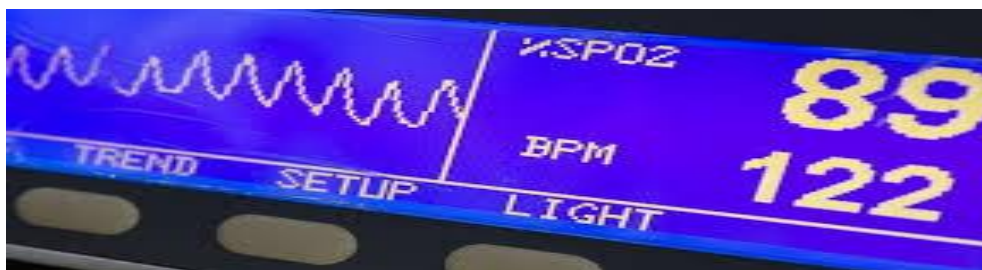
Figure 10: Pulse oximeter showing a good plethysmographic (pulse) wave and low oxygen saturation
